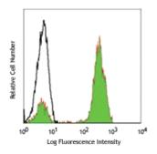
Typical results from human peripheral blood lymphocytes stained either with SK7 FITC used at 5  $\mu$ L/test (filled histogram) or with isotype control (open histogram).
